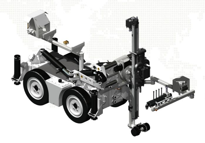
The CMAC PLH is a pneumatic/hydraulic drilling rig for production long-hole drilling and ground support applications for underground mining. The CMAC PLH is a popular pneumatic drill used for long-hole drilling in narrow-vein underground operations.
